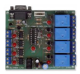
PIC-IO Firmware is an application developed by Goldtronica that allows galvanic and opto-isolated I/O interface from a RS232 port.
